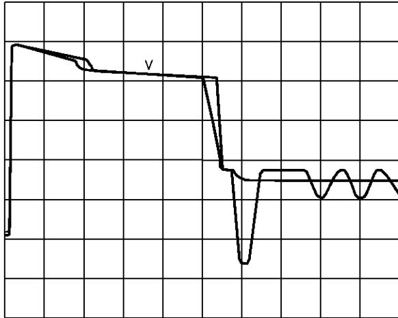
Figure 22 : Effect of Resistor in Parallel connected to the Yoke V = 10V/div.
